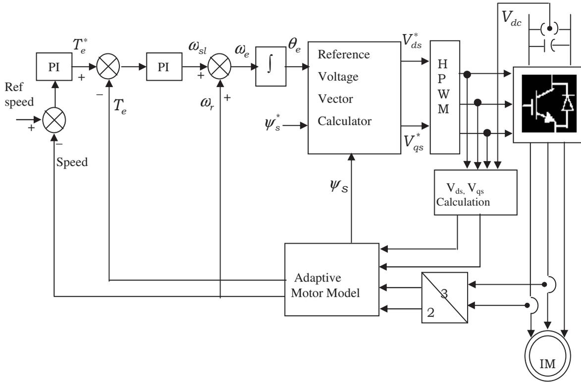
Fig. 8. Block diagram of proposed HPWM based DTC
