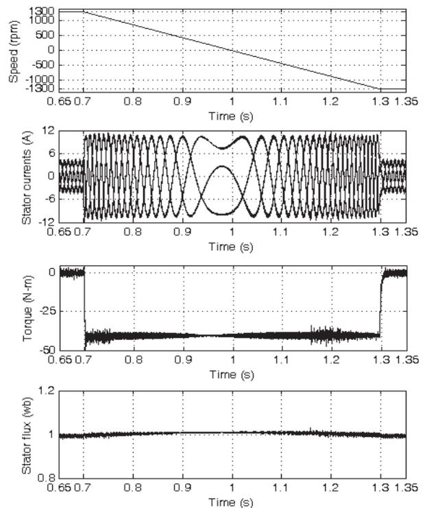
Fig. 16 transients during the speed reversal (speed is changed from +1300 rpm to -1300 rpm) for the proposed HPWM based DTC.
