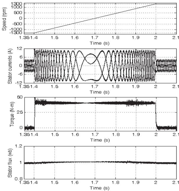
**Fig. 17. transients during the speed reversal (speed is changed from -1300 rpm to +1300 rpm) for the proposed HPWM based DTC**
