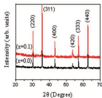
Figure 1. XRD patterns of  $\text{MgGd}_x\text{Fe}_{2-x}\text{O}_4$  ( $x=0.0$  &  $0.1$ )
