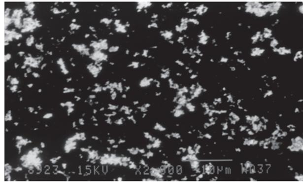
Figure 2. SEM of MgGd<sub>0.1</sub>Fe<sub>1.9</sub>O<sub>4</sub> powder sintered at 1000°C
