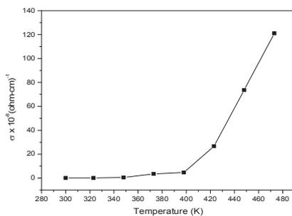
Figure 3. Variation of electrical conductivity of MgGd<sub>0.1</sub>Fe<sub>1.9</sub>O<sub>4</sub> ferrite with temperature
