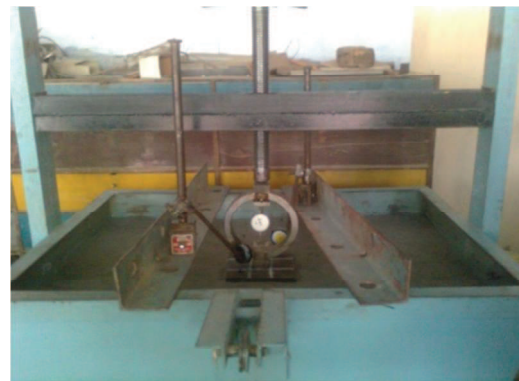
Fig. 4. Plate Load Test Setup
