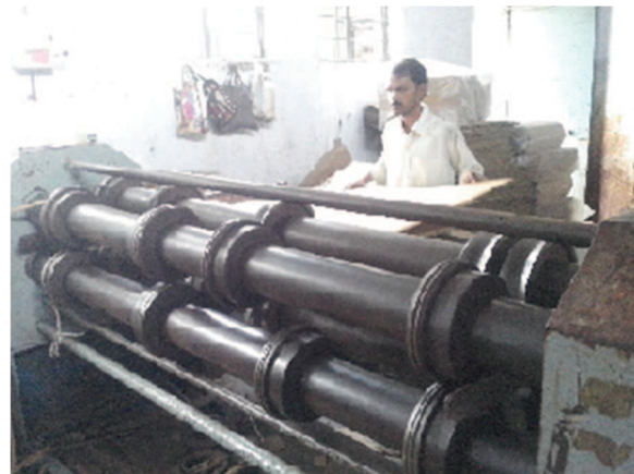
Figure 2.3 Process of creasing
