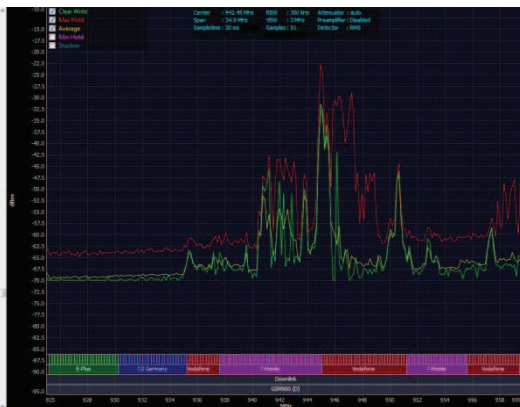
Fig. 3 : Frequency spectrum of GSM 900 taken in BVT
