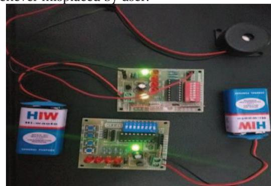
Fig.6 Interfacing of RF module along with Buzzer
