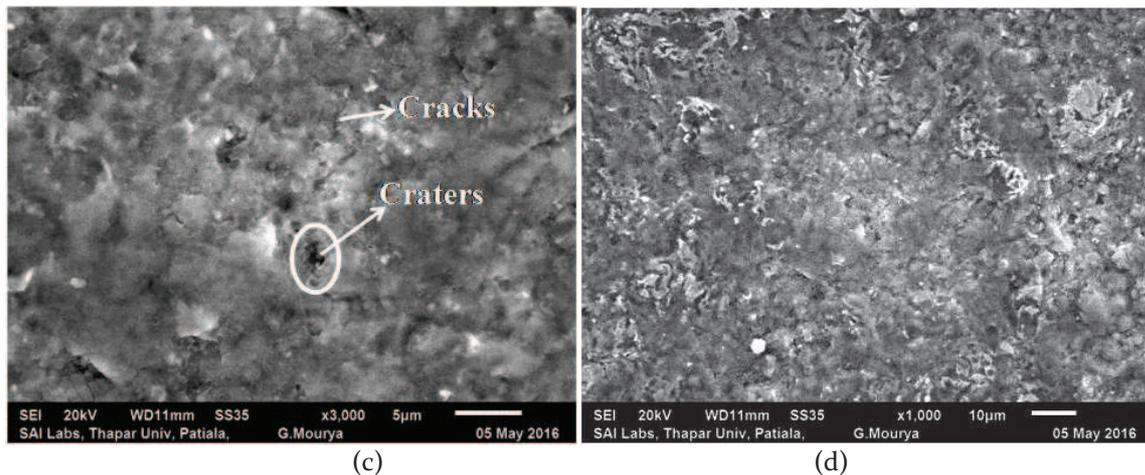
**Figure 5 SEM micrographs of untreated sample(a,b) and cryogenated treated samples(c,d) observed with Cracks, Craters and Debris at higher pulse on time = 120  $\mu$ s, pulse off time = 50  $\mu$ s, Spark gap voltage= 60 V and Wire feed= 5 m/min**
