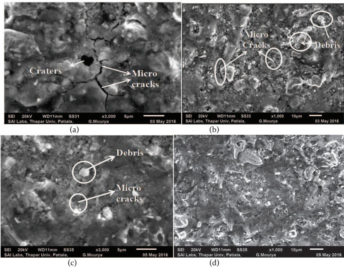
**Figure 4 SEM micrographs of untreated sample(a,b) and cryogenated treated samples(c,d) observed with Cracks, Craters and Debris at higher pulse on time = 120 µs, pulse off time = 45 µs, Spark gap voltage= 50 V and Ra= 2.36 µm. (Source: Sai Labs, Thapar University, Patiala)**
