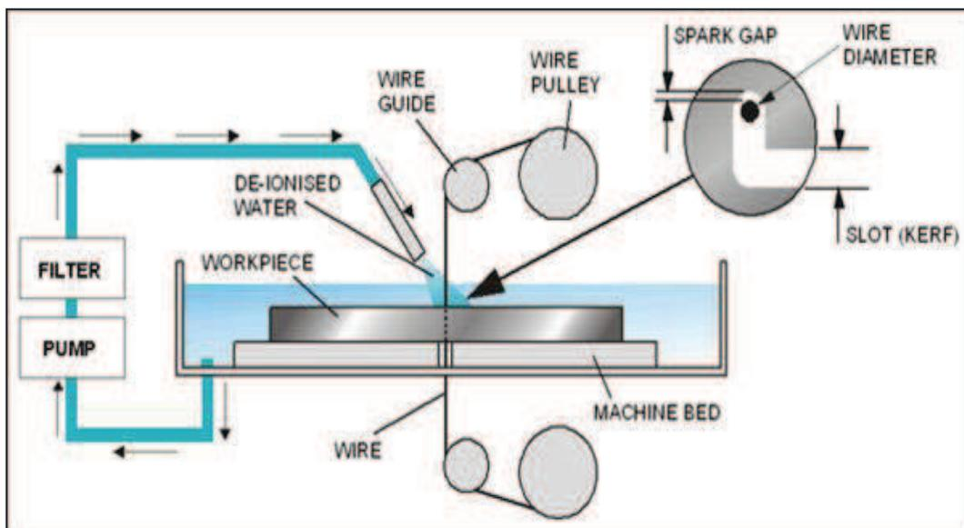
Fig 1. Schematic diagram of WEDM system (Guitrau, 1997)[4]
