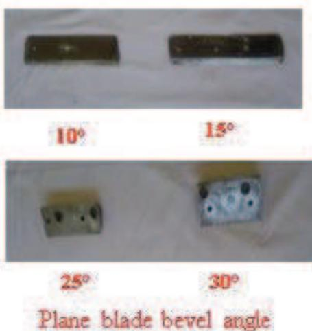
**Plate 1 Cutting blades of different angles**
