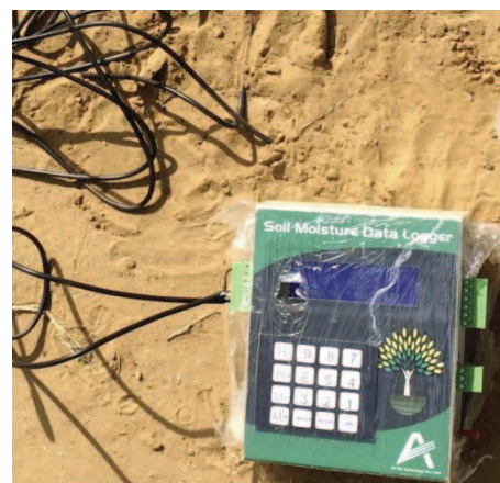
Fig. 2 Soil Moisture Data Logger
