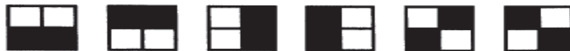
Horizontal transparencies vertical transparencies diagonal transparencies Figure-1: Six possible patterns of sub-pixel arrangements with 50% gray. Each pattern is represented as [0 0 1 1], [1 1 0 0], [0 1 0 1], [1 0 1 0], [0 1 1 0], [1 0 0 1] from left to right.
