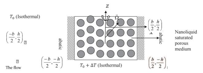
is governed by the Brinkman model with effects of Coriolis force and centrifugal acceleration included where centrifugal term is absorbed in pressure term of the linear momentum equation. An appropriate single-phase equations with suitable correction for a rotating porous medium is used [6]. The non-dimensional form of governing equations are:
