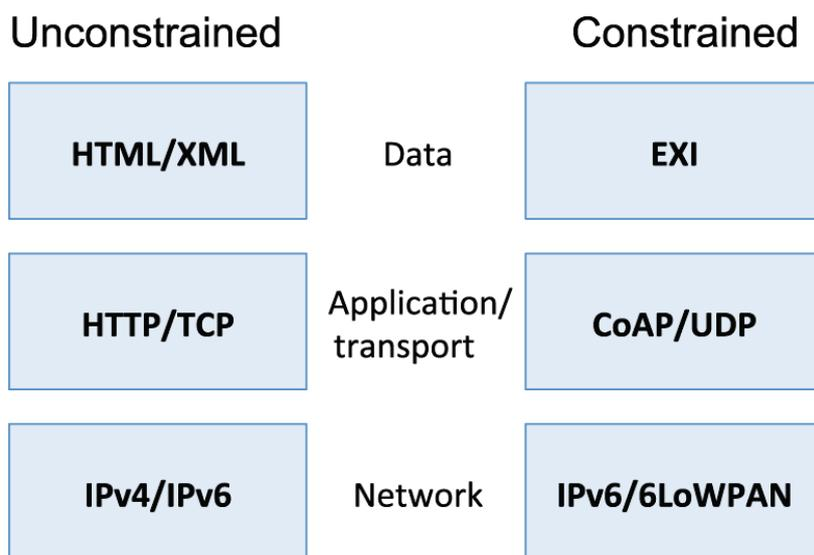
Fig 3: Protocol Stacks for constrained and unconstrained IOT nodes.
