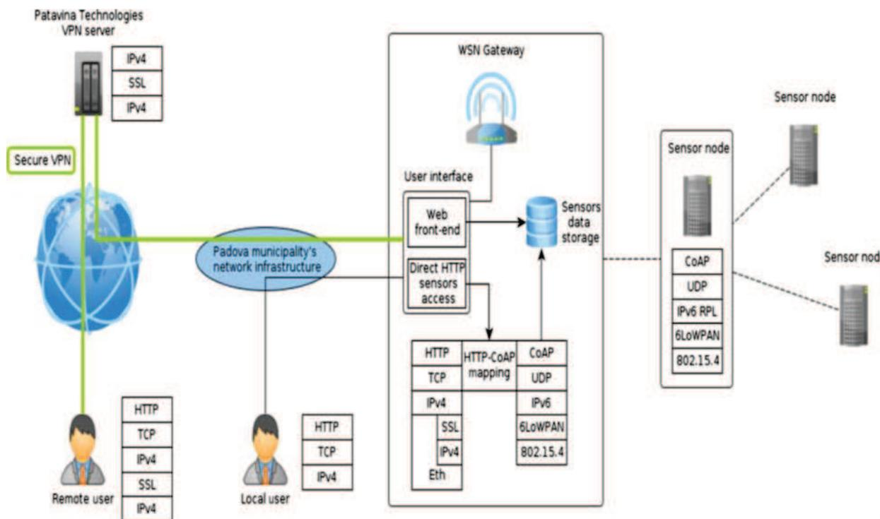
Fig 2: System architecture of smart city
