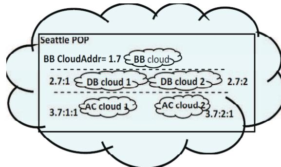
*Fig 2: Tiered Addresses in an ISP POP; BB=Backbone,DB=Distribution,AC=Access*
