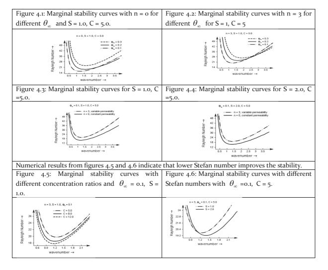
**Conclusion**: The linear stability is enhanced by smaller values of C for fixed S and far field temperature. It is also observed that higher far field temperature enhances the linear stability.
