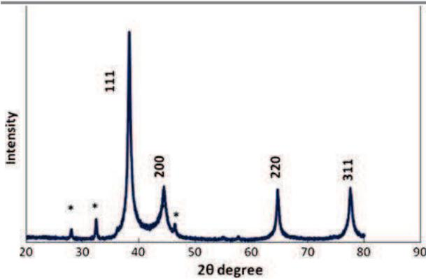
**Fig.3:** XRD pattern of silver nanoparticles green synthesized by lemon grass extract.
